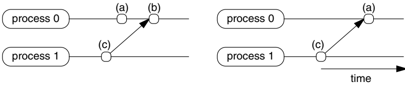
Fig. 2. Nondeterministic nonblocking receive/test operations on process 0.
